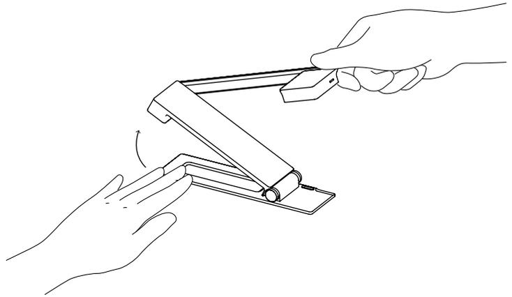
2. Press against the base plate of DO-CAM and pull it up.
