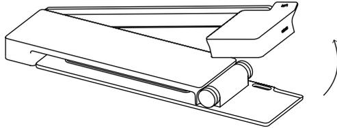
1. Start by lifting the camera head.
